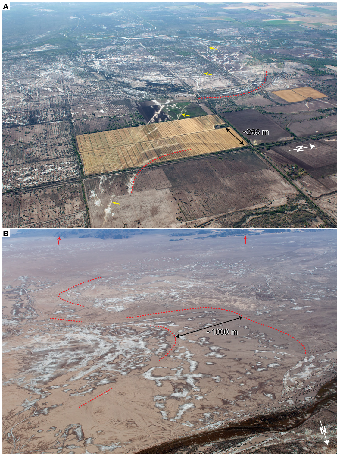
Figure 4. Oblique aerial photos of El Mayor–Cucapah (EMC) rupture in the Delta domain (photo locations plotted in Fig. 3). (A) Northwest-striking tectonic scarps (yellow arrows) cut across abandoned and buried meanders (red dashed lines) of the Colorado River delta. White deposits are coseismic sand blows that erupted along tectonic fractures and buried sandbars. Photo azimuth is \sim 285^\circ . (B) White deposits generated by dewatering and liquefaction are observed throughout the southern Colorado River delta and extend to the margin of the Sierra Pintá (red arrows), which is more than 12 km from the main zone of tectonic surface rupture (Fig. 3). Prominent fractures along the axis of the elongated sand blow deposits curve and follow abandoned and buried meanders (red dashed lines). Photo azimuth is \sim 190^\circ . Photos taken by John M. Fletcher. See Supplemental Files 1 and 2 (see footnotes 1 and 2) for photo information in Google Earth KMZ format and Microsoft Excel table format, respectively.
